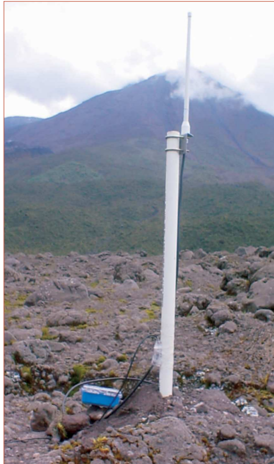
Figure 2. A two-component station. The blue Pelican case contains the wireless sensor node and hardware interface board. The external antenna is mounted on the PVC pole to reduce ground effects. A microphone is taped to the PVC pole, and a single seismometer is buried nearby.
